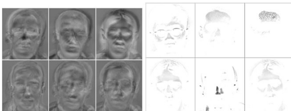
Figure 1.2: Facial image recognition - PCA vs NMF - In this example the basis components extracted with PCA (left panel) and those with NMF (right panel) for 6 images of faces are compared. The eigenfaces obtained by PCA are prototypical faces containing all kinds of facial traits, while the NMF basis vectors represent particular traits: different kind of eyes, noses, and mouths (from Naik, 2015).
