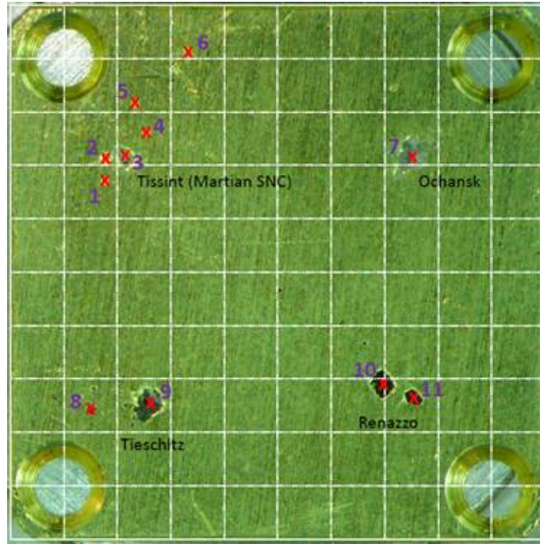
Figure 4.2: Target 4E1 - Image of Target 4E1 (gold plate) with eleven corns placed upon it. The corns belong to different classes, taken from CoMeCS-Project (2017).
