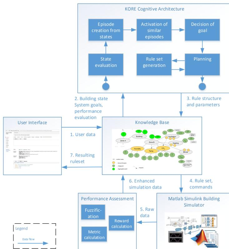
The method used for optimization is **reinforced learning combined with case-based reasoning**. The system tests different solutions, evaluates and stores the evaluation of the solutions in a knowledge base. Since it receives constantly feedback for its decisions, its strength lies in the ability to adapt to dynamic changing environments.
