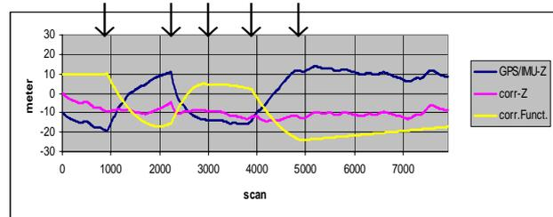
Figure 2: Z-correction by drift-modelling for str.17: **GPS/IMU-Z**: original GPS/IMU-Z-values / **corr.Funct.**: correction function (determined in the adjustment) / **corr-Z**: corrected Z-values after applying of the corr.Funct. / ↓: sites of breaking up the GPS/IMU-model of str.17.
