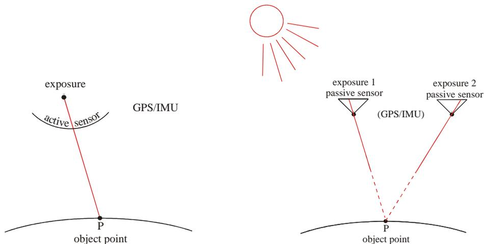
Figure 1: Paradigm of laser scanning    Figure 2: Paradigm of Stereo-Photogrammetry
