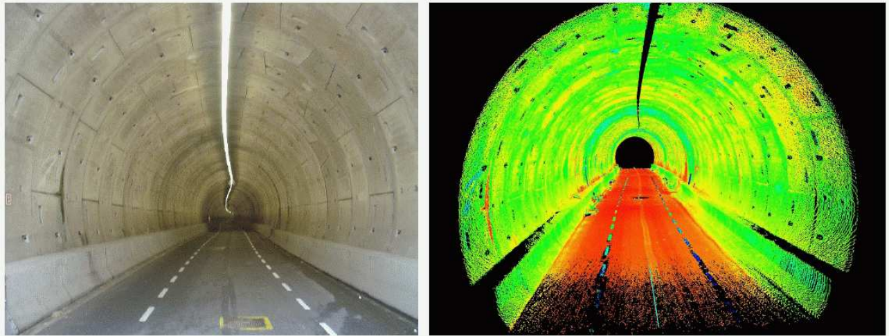
Figure 3. Left: photograph of the 2e Heinenoordtunnel. Right: laser scan, colored by intensity, from red to blue. Clearly visible is the low reflectivity of the asphalt in contrast to the high reflectivity of the road markers.
