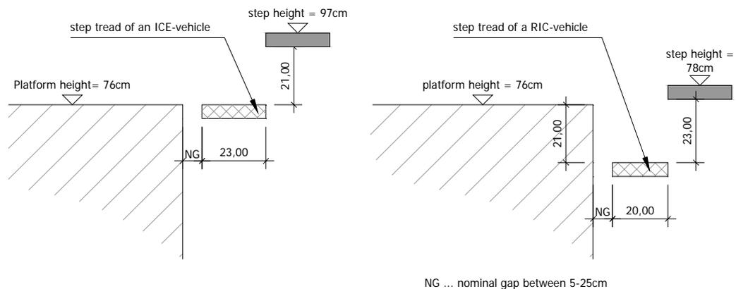
**Figure 2.** Gap between an ICE and platform with a height of 76cm (left)
