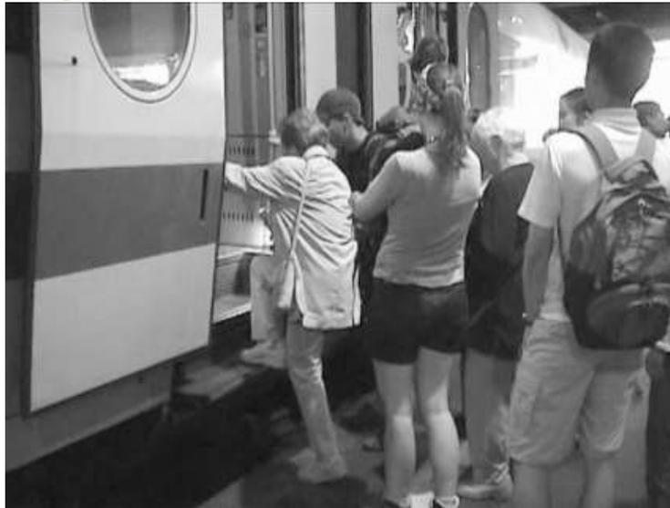
Figure 1. Boarding passenger onto an ICE on a platform height of 38cm
