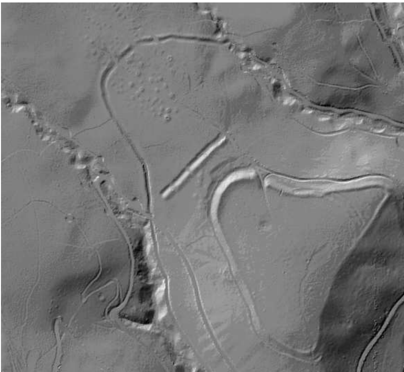
Fig. 8 - Shading of the resulting digital terrain model of an Iron Age hillfort in the Leitha mountain range after the process of fine geo-referencing and advanced classification using the additional full-waveform information.
