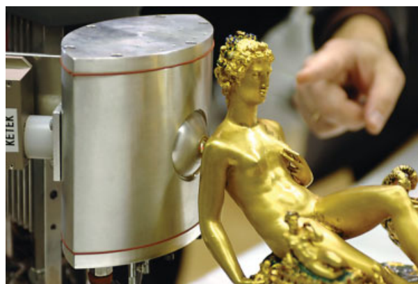
Figure 3. The vacuum chamber of the ( \mu -) XRF instrument. The Kapton ® window is located 1–2 mm from the investigated object. Photo Credit: D.Calma/IAEA.
