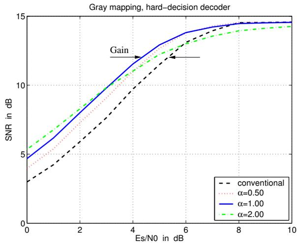
Fig. 6. System performance in terms of source SNR using energy allocation by  $S$ -values with  $\alpha = \{0.5, 1.0, 2.0\}$ ; comparison with a conventional system; Gray mapping. A conventional hard-decision receiver was always used.
