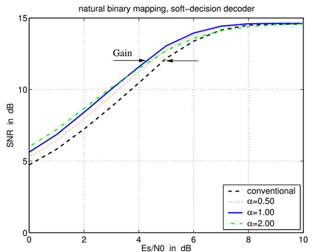
Fig. 9. System performance in terms of source SNR using energy allocation by  $S$ -values with  $\alpha = \{0.5, 1.0, 2.0\}$ ; comparison with a conventional system; natural binary mapping. A conventional soft-decision receiver was used.
