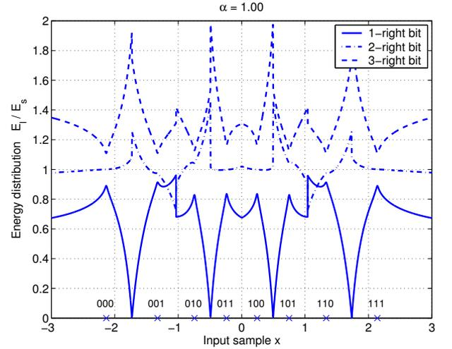
Fig. 5. Energy distribution according to (13) with  $\alpha = 1.00$  based on the  $S$ -values in Fig. 3 (natural binary bit mapping).
