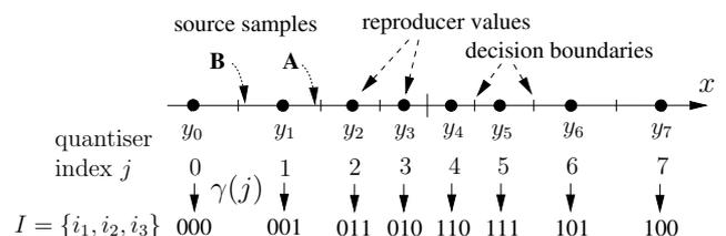
Fig. 1. Three-bit scalar quantiser with Gray bit-mapping  $\gamma()$ .
