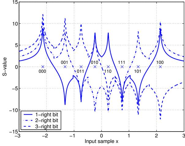
Fig. 2.  $S$ -values for a three-bit scalar Lloyd-Max quantiser for a Gaussian source; Gray bit mapping;  $\beta = 10^{-4}\sigma_x^2$  in (2); the quantiser reproducer values are marked by “ $\times$ ”, the bit mapping is included as well.
