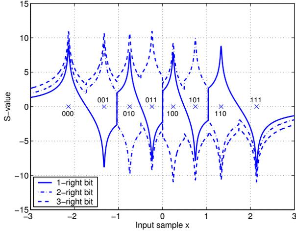
Fig. 3.  $S$ -values for a three-bit scalar Lloyd-Max quantiser for a Gaussian source; natural binary bit mapping;  $\beta = 10^{-4}\sigma_x^2$  in (2); the quantiser reproducer values are marked by “ $\times$ ”, the bit mapping is included as well.
