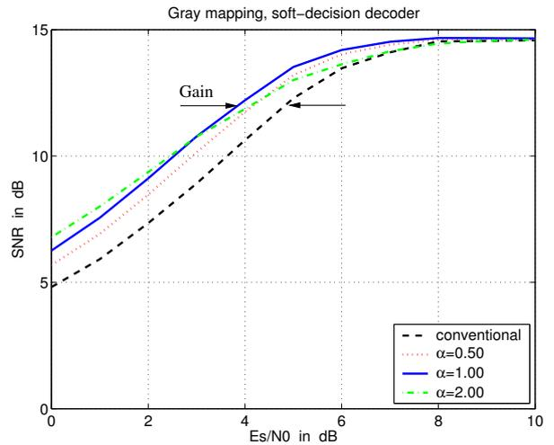
Fig. 8. System performance in terms of source SNR using energy allocation by  $S$ -values with  $\alpha = \{0.5, 1.0, 2.0\}$ ; comparison with a conventional system; Gray mapping. A conventional soft-decision receiver was always used.
