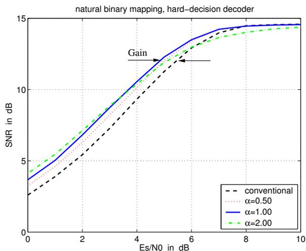
Fig. 7. System performance in terms of source SNR using energy allocation by  $S$ -values with  $\alpha = \{0.5, 1.0, 2.0\}$ ; comparison with a conventional system; natural binary mapping. A conventional hard-decision receiver was used.
