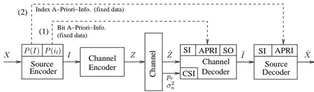
Fig. 4. (1) Channel decoding aided by residual redundancies and (2) estimation-based source decoding
