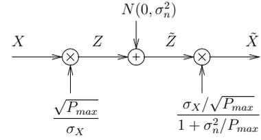
Fig. 2. Optimal encoder-decoder pair for the transmission of a Gaussian source over a Gaussian channel with average input power constraint.
