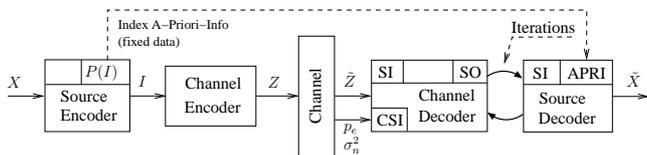
Fig. 5. Iterative source-channel decoding
