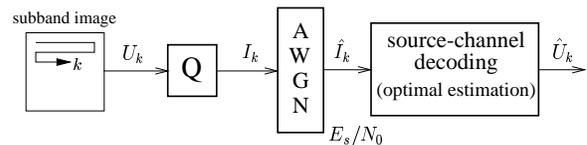
**Figure 1. Simple model of the transmission system**
