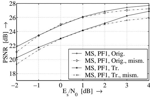
**Figure 6. Performance under channel mismatch conditions ("mism."), and comparison to the matched case ( $R = 0.36$  bpp,  $L = 3$ ). The decoder is designed for a fixed channel-SNR of  $E_s/N_0 = 1$  dB.**
