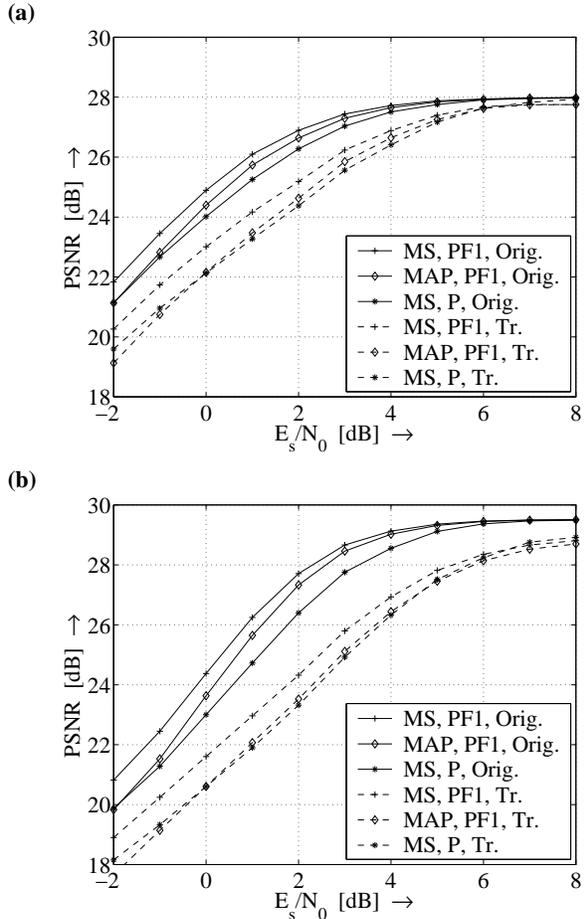
**Figure 5. Performance using different methods for representing the transition probabilities at the decoder ( $R = 0.36$  bpp,  $L = 3$ ): (a) "Goldhill", (b) "Lena" image.**
