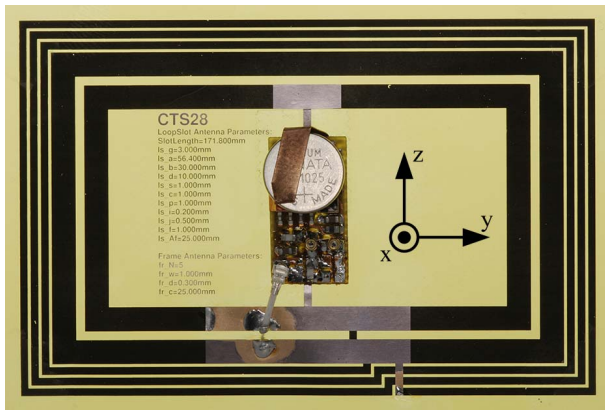
Fig. 5. Dual-band tag antenna prototype with battery driven oscillator.
