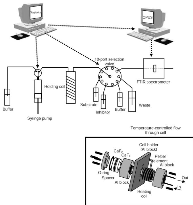
FIG. 1. Scheme of the experimental setup consisting of an automated flow system and a temperature-controlled mid-infrared flow-through sensor containing AChE immobilized on agarose beads.
