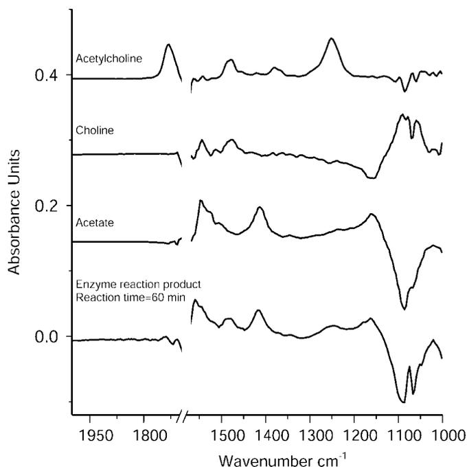
FIG. 2. Absorbance spectra of (top to bottom) 4 g L<sup>-1</sup> acetylcholine standard, 2 g L<sup>-1</sup> choline standard, 2 g L<sup>-1</sup> acetic acid (acetate), and enzyme reaction products after a batch reaction time of 1 hour. Spectra were obtained using 128 co-added scans, 8 cm<sup>-1</sup> nominal resolution, and 0.1 M phosphate buffer as background. Note: Spectra were shifted on the y-axis for clarity.
