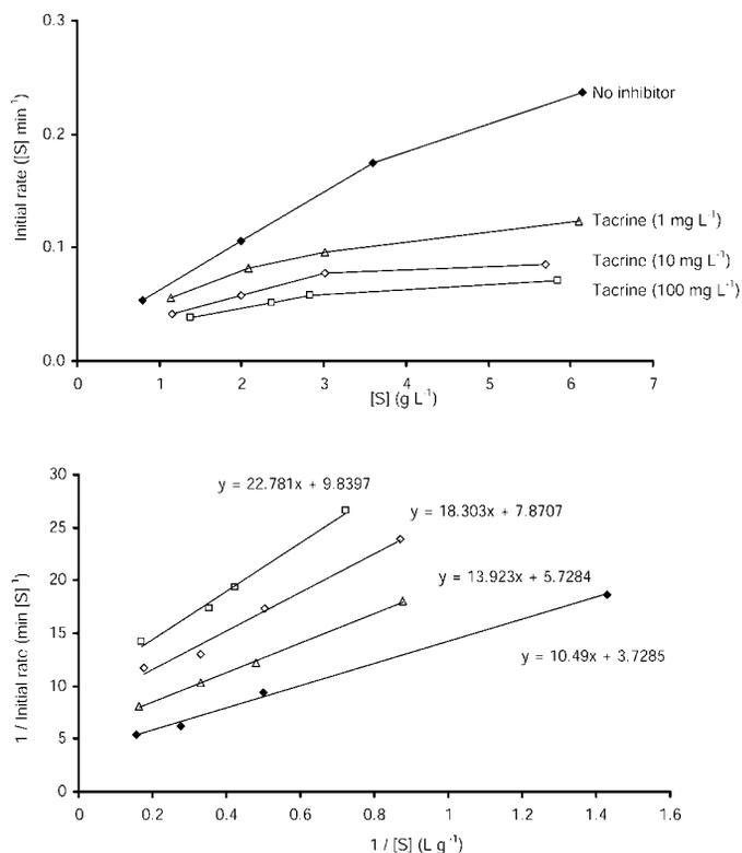
FIG. 4. (Top) Inhibition of the hydrolysis of ACh by tacrine at different concentrations. (Bottom) Lineweaver–Bulk plot of initial reaction rates against AChE concentration in the presence (at different concentrations) and absence of tacrine.
