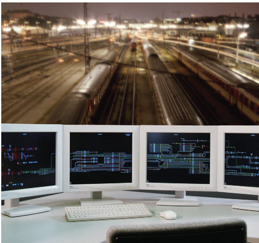
Figure 1: Electronic interlocking for mainline rail.
