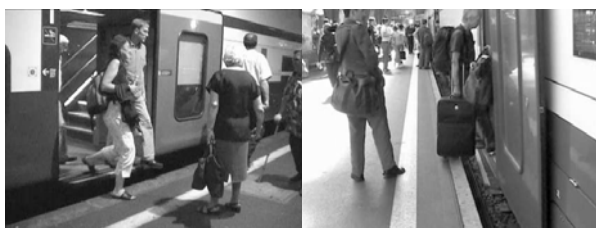
Figure 6 IC2000 on a platform height of 38cm (left) IC 2000 on a platform height of 55cm (right)
