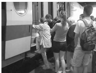
Figure 1 Boarding passenger onto an ICE on a platform height of 38cm
