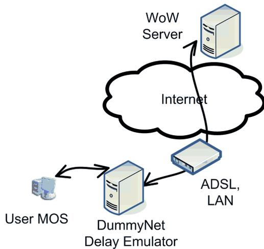
Figure 1: Measurement setup with additional delay.
