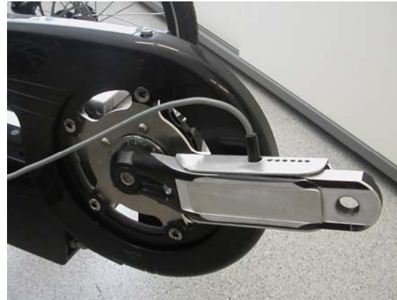
Fig. 3: Right force measurement crank with removed pedal and orthosis. (Displayed cable for battery charging)
