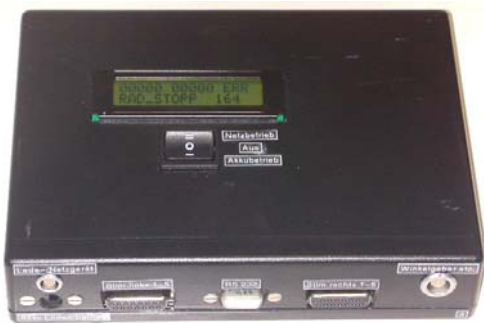
Fig. 2: Current controlled 10-channel stimulator: induces biphasic rectangular pulses with a stimulation current from 0-150 mA (at 1 k \Omega ), frequency from 0-100 Hz, and pulse width from 0-700 \mu s
