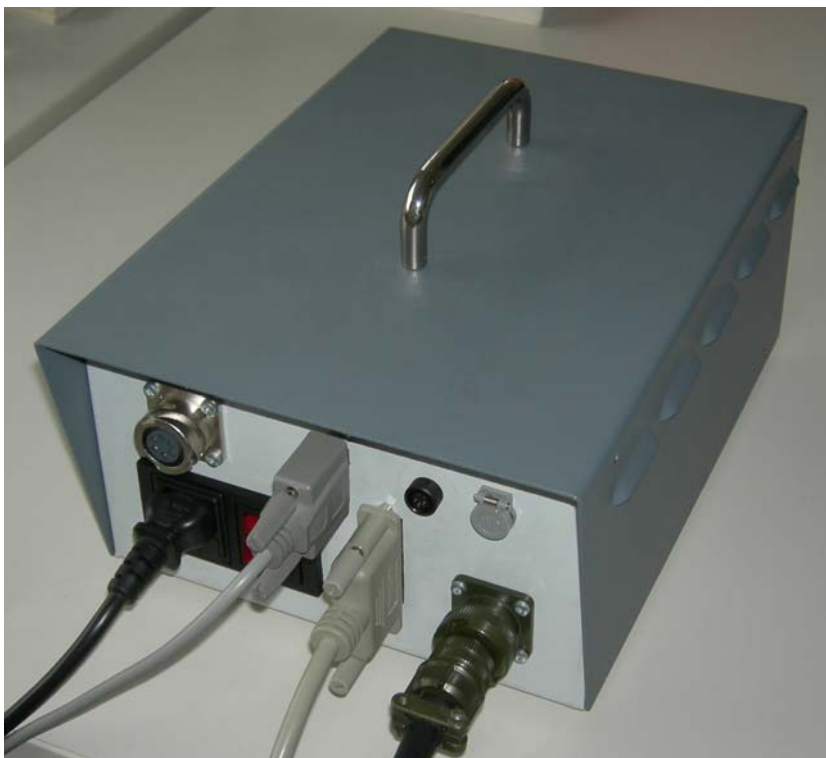
Fig. 3: The controller box (dimensions 250x200x120mm) including an on/off switch, a device fuse and connectors to the drive-train (power and data separated), the stimulator, the emergency stop button, the handheld stimulation intensity controller and the 230V~ electricity network.
