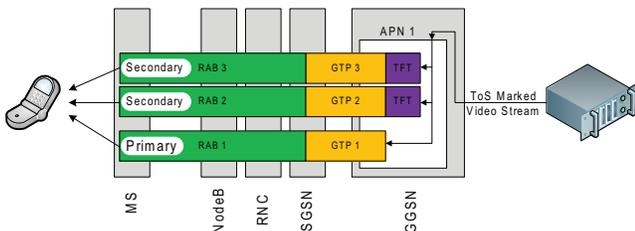
Fig. 5. Routing of QoS oriented data originating from one application server.
