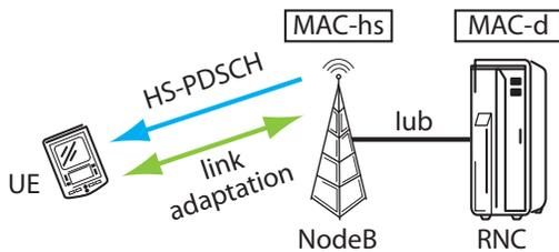
Fig. 1. Main physical layer associated network elements of HSDPA. The fast link adaptation (TTI based) is terminated at the NodeB.
