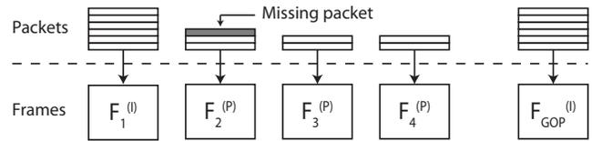
Fig. 3. Temporal dependency of encoded frames
