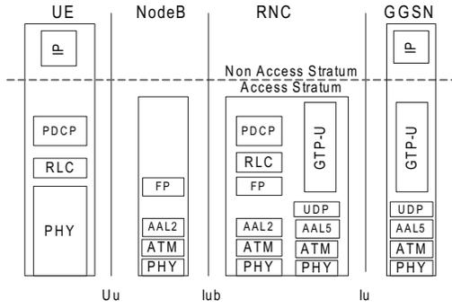
Fig. 4. UMTS Protocol Stack (User Plane).
