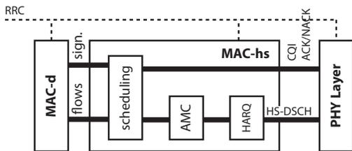
Fig. 2. Overview of the layer interaction responsible for the physical layer transmissions in HSDPA.
