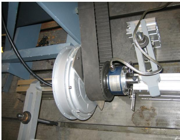
Fig. 2. Picture of the used outer-rotor PMSM with encoder and load-machine
