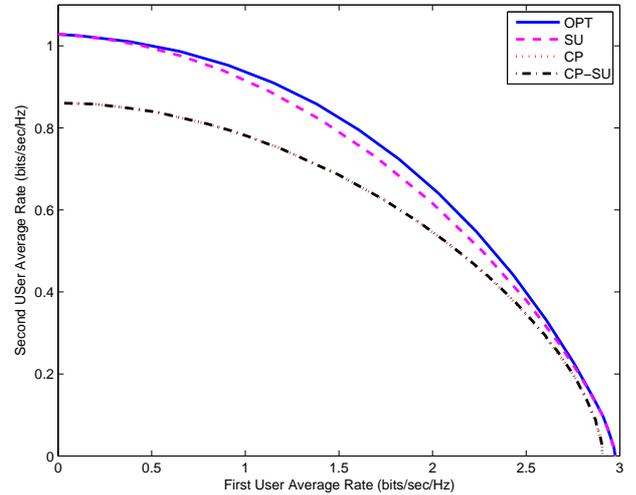
Fig. 1. Boundaries of the ergodic capacity regions for the two-user case. The users are Rayleigh-faded with 10dB difference in average channel qualities.
