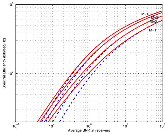
Fig. 2. Differences in spectral efficiency between optimal power control (solid lines) and constant power per block (dashed lines) for different number of users  $M$ . Rayleigh fading channels with identical long-term average channel qualities. Maximum sum-throughput is considered.
