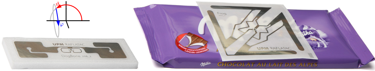
Fig. 2. UPM Dogbone transponder (left) and UPM Frog transponder on a bar of chocolate (right). The photographs are shown with the coordinate system used for characterization of the antennas.
