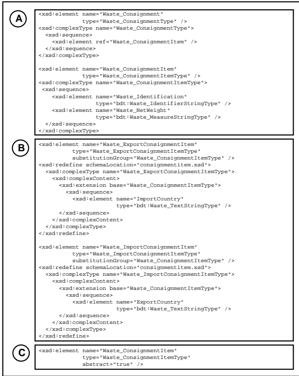
Figure 8: Substitution Group Mechanism (1/3).
