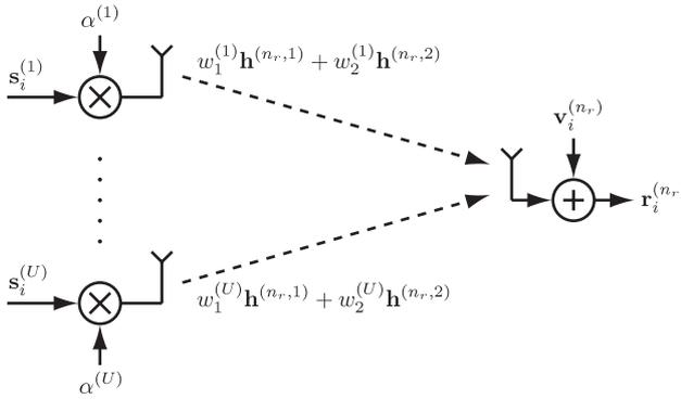
Fig. 2. Equivalent representation of the multi-user TxAA transmission, representing  $U$  virtual antennas and  $U$  virtual channels.
