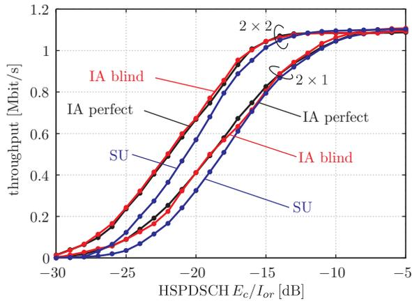
Fig. 6. Throughput of desired user in a spatially uncorrelated ITU PedA channel at CQI 13, corresponding to a maximum throughput of 1.14 Mbit/s.
