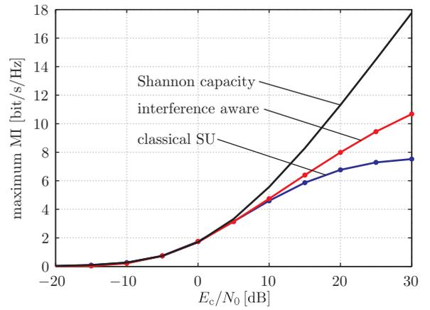
Fig. 4. Comparison of the maximum MI performances of the classical SU equalizer and the proposed interference-aware equalizer when assuming Gaussian post-equalization interference.
