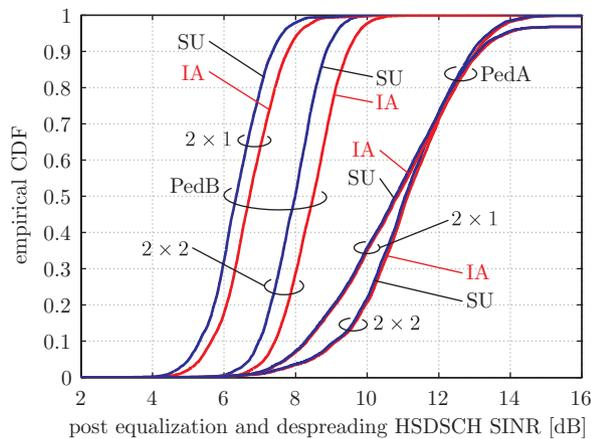
Fig. 8. Empirical CDFs of the post equalization and despreading SINR of the HS-DSCH.
