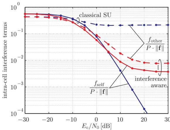
Fig. 3. Intra-cell interference terms  $f_{\text{self}}$  and  $f_{\text{other}}$  for the classical SU equalizer and the proposed interference-aware equalizer, assuming perfect knowledge of the cell's pre-coding state.
