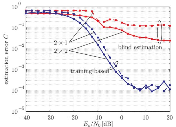
Fig. 5. Estimation error  $C$  of the LS and the second-order blind estimator versus  $E_{\text{c}}/N_0$ , see Equation (24).
