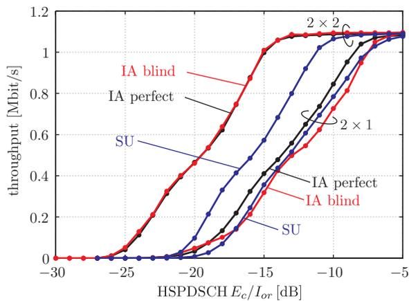
Fig. 7. Throughput of desired user in a spatially uncorrelated ITU PedB channel at CQI 13, corresponding to a maximum throughput of 1.14 Mbit/s.
