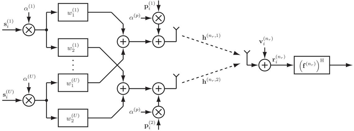
Fig. 1. Multi-user transmission in TxAA, for a total number  $U$  of simultaneously served users. The pre-coding is conducted individually for every user. At the receiver, only one receive antenna is depicted, although the scheme allows for an arbitrary number of receive antennas.
