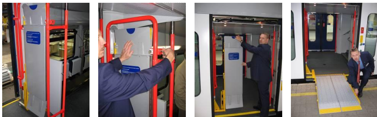
Ramp in vehicle.
