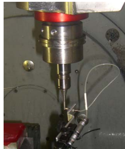
Fig. 2. Ultrasonic tool with measurement device
