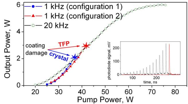
Fig. 3. (Color online) Dependence of the output power on the incident optical pump power in the CPA regime. Solid circles and triangles correspond to two different cavity configurations, described in the text, at the repetition rate of 1 kHz and 90 cavity round trips. Open circles show the performance at 20 kHz. Inset, oscilloscope traces of the intracavity pulse train (dashed curve) and the selected pulse (solid curve) taken at the 3 mJ output energy.
