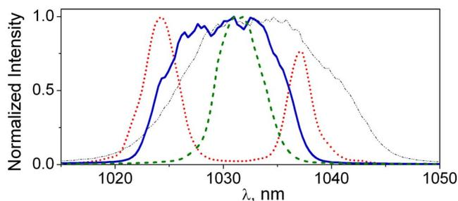
Fig. 4. (Color online) Spectra of the seed laser before (thin dotted curve) and after (thick dotted curve) shaping; resulting spectra of the RA output without (dashed curve) and with (solid curve) shaper installed.
