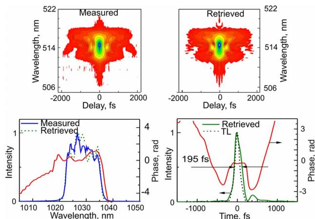
Fig. 5. (Color online) Recompressed pulse measurement with SHG FROG for the output energy of 1 mJ. TL represents the transform-limited pulse.
