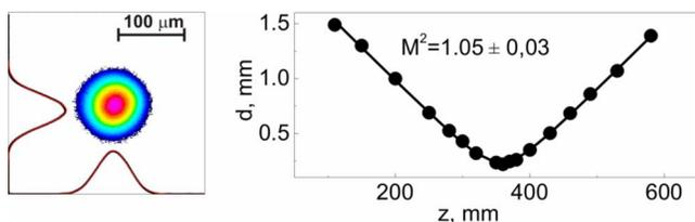
Fig. 2. (Color online) Left, profile of the 1 mJ 1 kHz output beam in the focus of a lens ( $f = 300$  mm); curves, vertical and horizontal beam profile cross sections. Right,  $M^2$  measurement; dots, experimental data; solid curve, a fit corresponding to an  $M^2$  of 1.05.
