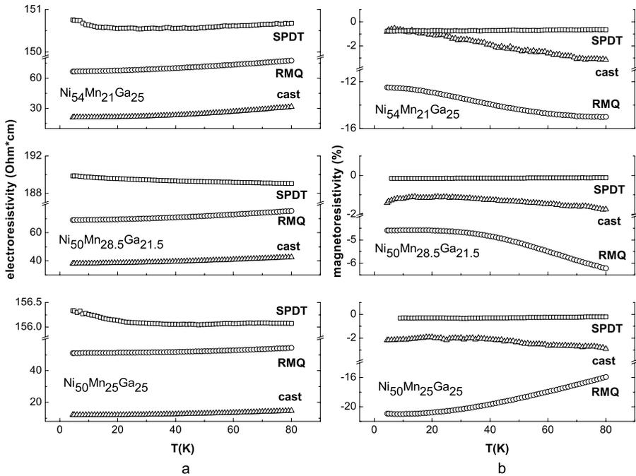
**Fig. 1** Temperature dependence of the electro- and magnetoresistivity in a field of 10 T for Ni-Mn-Ga alloys
