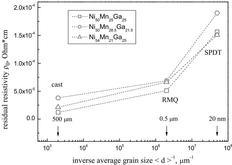
**Fig. 2** “Size” dependence of the residual resistivity for Ni-Mn-Ga alloys
