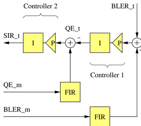
Fig. 6. New OLPC alg. using uncoded BER information
