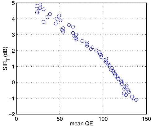
Fig. 3. Measured target SIR over mean QE, single connection
