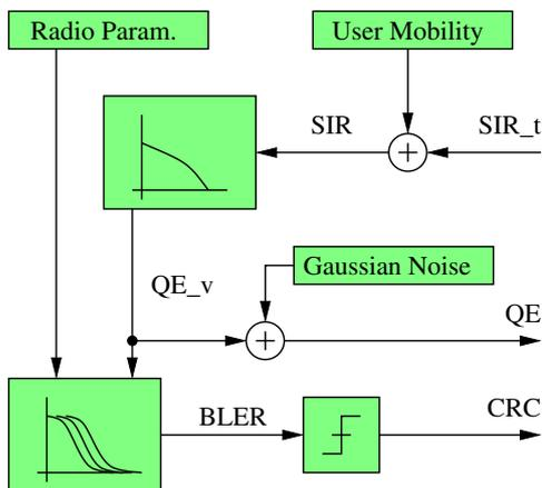
Fig. 5. Model of the control path of the OLPC
