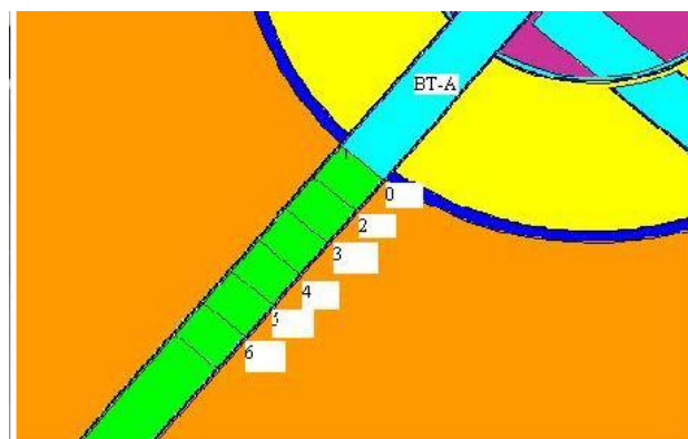
Figure 4: MCNP (YZ-view) of beam tube A
