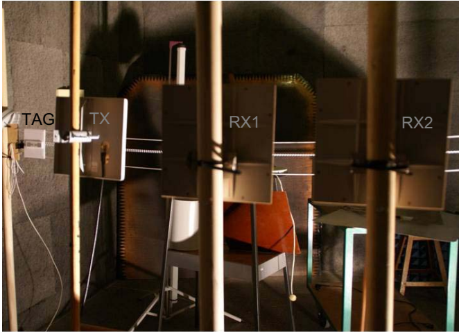
Figure 4: Measurement setup with TX (left) and RX (right) antennas. The tag is moved on the motor driven nylon cord through the measurement room. The fading in the room is generated artificially by placing one dominant ( \approx 2.5 \text{ m}^2 ) reflector in back left corner (position x=0 \text{ m} , y=0 \text{ m} ) and distributing several smaller reflectors in the measurement scenario.
