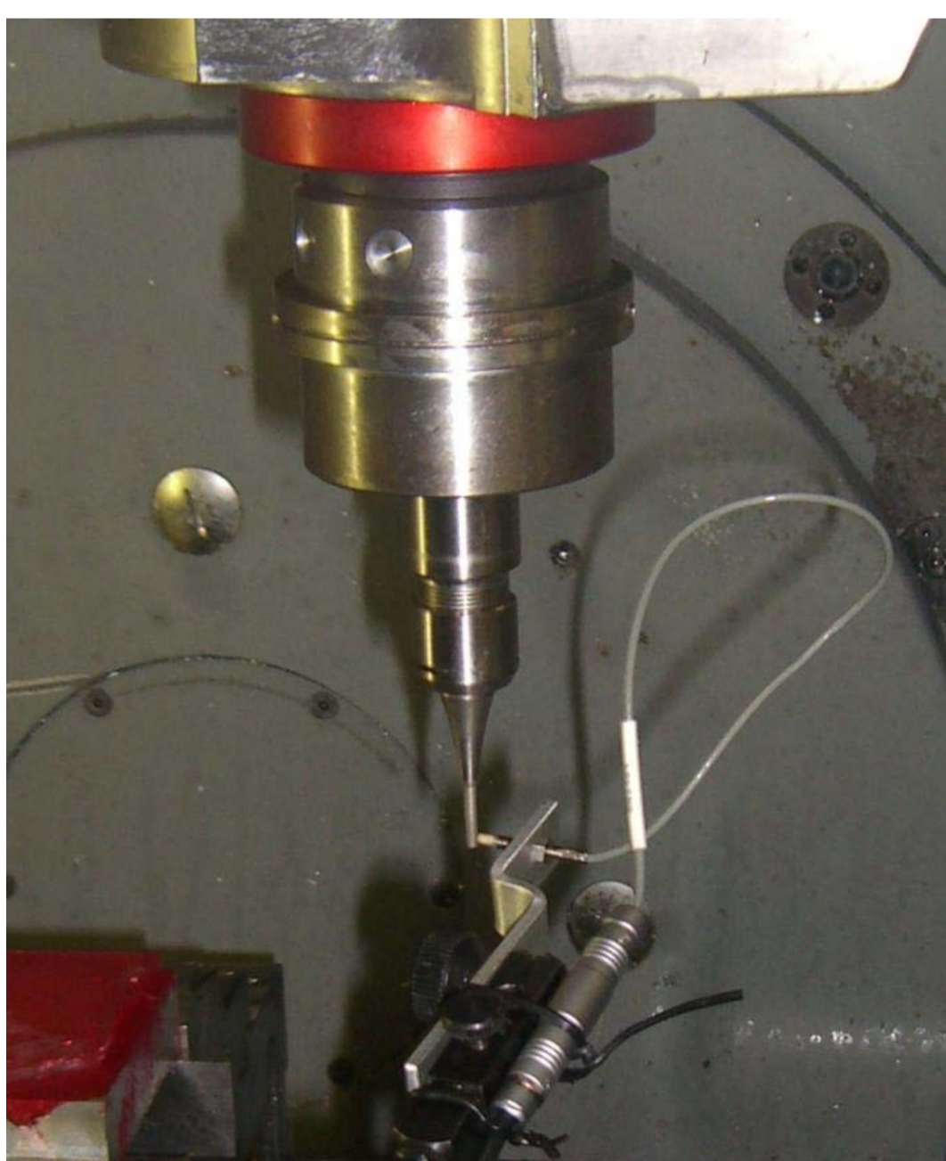
Fig. 2: Ultrasonic tool with measurement device
