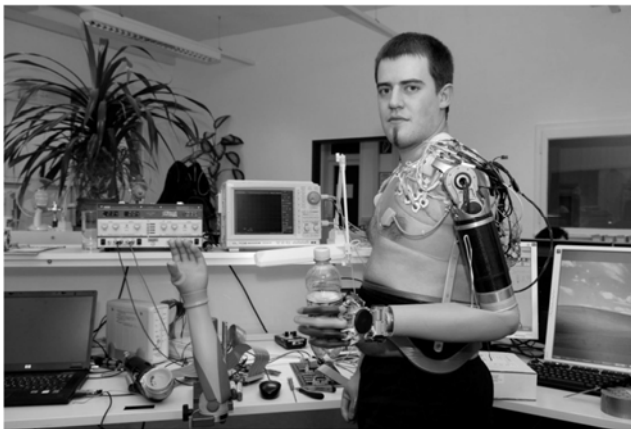
Figure 1: The first prosthesis developed by the company Otto Bock, global market leader in the area of prostheses which control the five fingers of the artificial hand as well as the hand itself via a complex nervous system. 2
