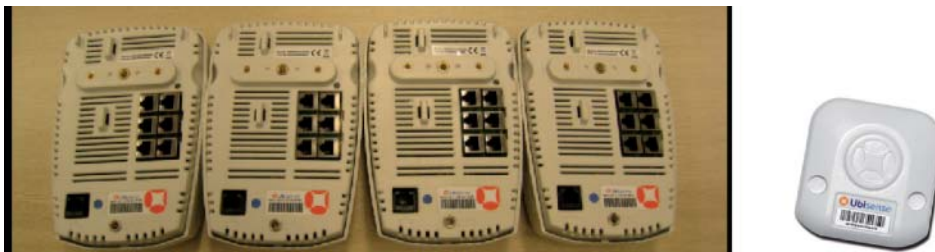
Figure 3: Ubisense UWB-AoA sensors (left) and a typical UWB-AoA tag (right).
