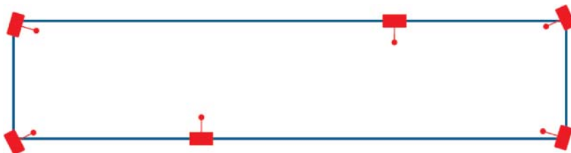
Figure 11: Sensor configuration suggested by Ubisense for UWB-AoA positioning in weak geometry areas.
