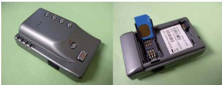
Figure 5: An example of low-cost GPRS enabled GPS tracker.
