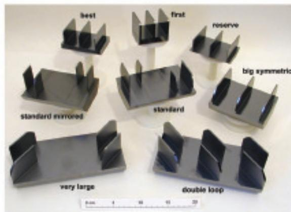
Fig. 2: (Top) Schematic sketch of a monolithic perfect crystal neutron interferometer. (Bottom) A collection of various types of interferometer crystals
