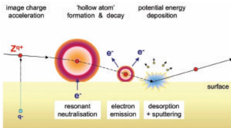
Fig. 3: Formation of 'hollow atoms' upon the interaction of slow highly charged particles with solid surfaces
