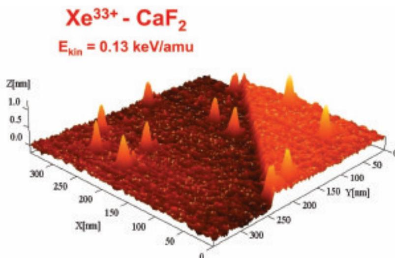
Fig. 4: Nano-sized modification of a CaF<sub>2</sub> surface upon bombardment with Xe<sup>33+</sup> ions
