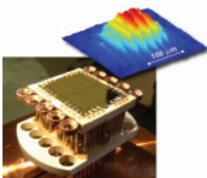
Fig. 9: The AtomChip technology allows the production and manipulation Bose-Einstein condensates. The enlarged 3D signature of a BEC is shown
