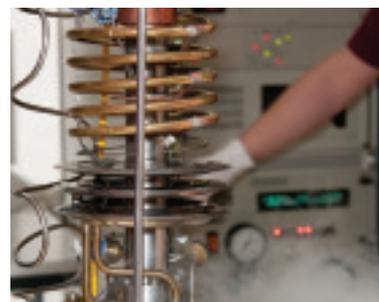
Fig. 7: Central part of a  $^3\text{He}-^4\text{He}$  dilution refrigerator at the IFP that cools samples down to about 10 milli-Kelvin prior to its combination with a nuclear demagnetisation stage with a base temperature in the micro-Kelvin range
