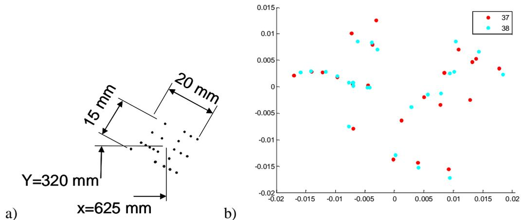
Figure 5: Relative Location of pencil lead breaks; a) pattern of pencil lead breaks; b) results from Relative Location processing
