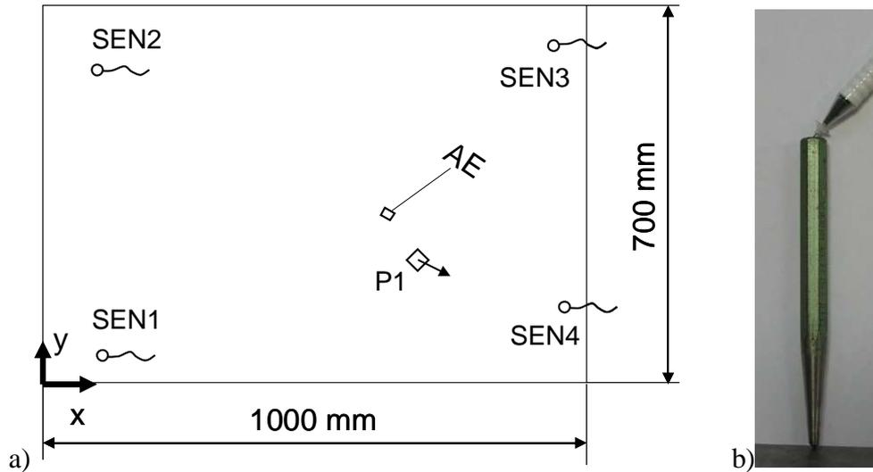
Figure 3: a) Arrangement for simple tests; steel plate with thickness of 6 mm; b) Pencil lead break via centre punch
