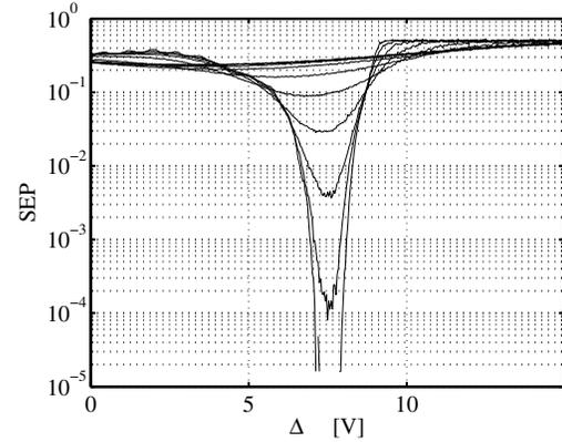
Figure 4. Sample of the Monte-Carlo optimization procedure for  $G_p=15$  dB and varying  $I/N$ .  $\text{SINR}_s=-15$  dB.
