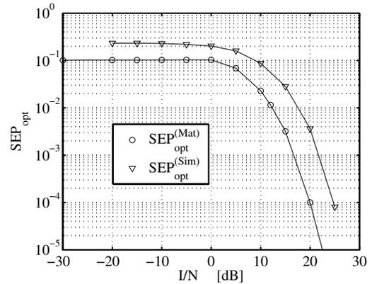
Figure 5. Static Analysis: Simulated and calculated optimum SEP in combined interference with  $G_p=15$  dB.  $\text{SINR}_s=-15$  dB.
