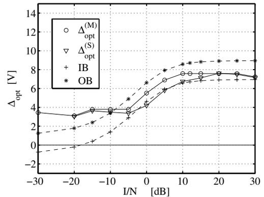
Figure 6. Static Analysis: Simulated and calculated optimum threshold locations in combined interference.  $\text{SINR}_s=-15$  dB.
