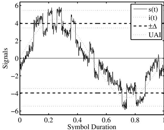
Figure 3. Sample of the investigated input signal (unfiltered). UAI ... unambiguous interval.
