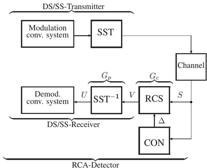
Figure 1. Structure of the investigated communication system. SST ... spread-spectrum technology, DS/SS ... direct-sequence spread-spectrum, RCS ... reliable chip selector, RCA ... reliable chip accumulator, CON ... control module,  $G_p$  ... processing gain,  $G_c$  ... conversion gain,  $\Delta$  ... threshold,  $S, V, U$  ... random variables.
