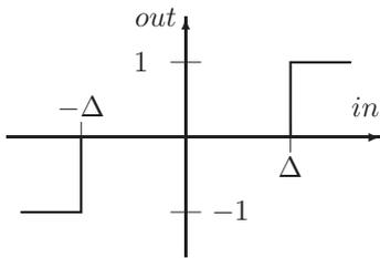
Figure 2. Transfer characteristic of the reliable chip selector.
