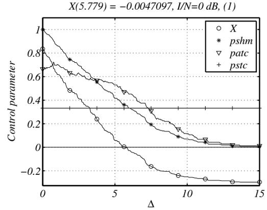
Figure 8. Sample of the control variable for I/N=0 dB and  $SINR_s=-15$  dB with  $k_p=1.44$ ,  $k_a=0.46$  and  $k_s=0.90$ .  $T_{ob} = 10 T_0$ .
