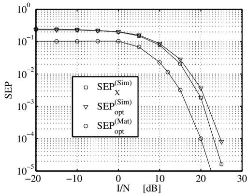
Figure 11. Comparison: Symbol error probability for combined interference.  $G_p=15$  dB and  $\text{SINR}_s=-15$  dB.
