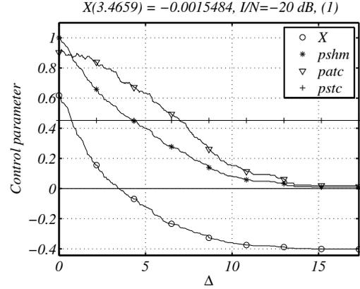
Figure 7. Sample of the control variable for I/N=-20 dB and  $SINR_s=-15$  dB with  $k_p=1.44$ ,  $k_a=0.46$  and  $k_s=0.90$ .  $T_{ob} = 10 T_0$ .
