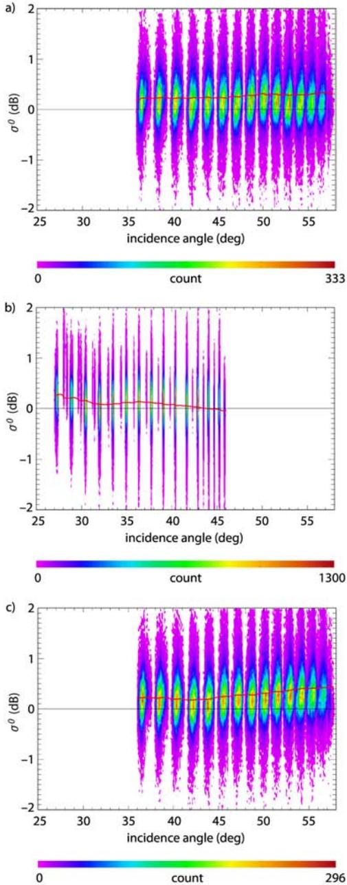
Figure 1. Collocated ASCAT – ERS-2  $\sigma^0$  differences according to incidence angle for a) fore, b) mid and c) aft beams. The red lines indicate moving average values with a window width of  $5^\circ$ .
