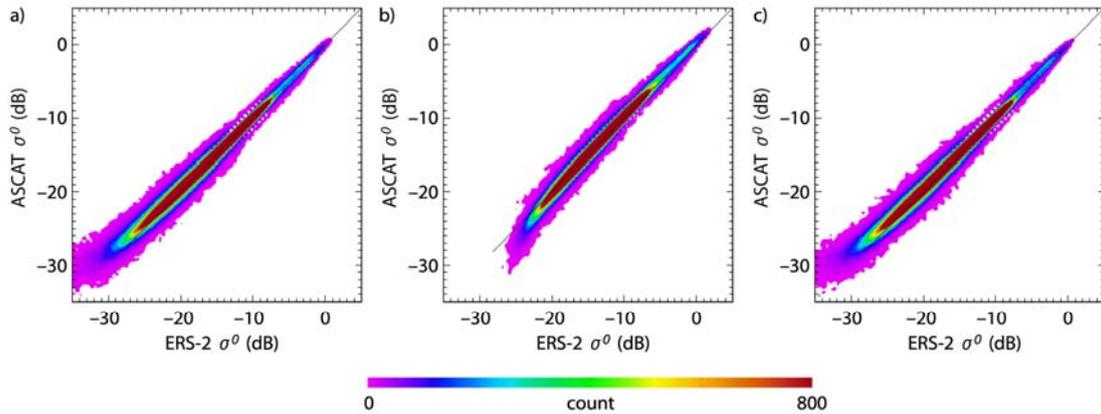
Figure 2. Collocated ERS-2 – ASCAT  $\sigma^0$  scatterplot for the a) fore-, b) mid- and c) aft beams.
