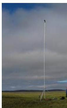
Figure 2. Samoylov Island, SPARC set-up for thermal upscaling: TIR camera mounted on 10 m mast, summer 2008.
