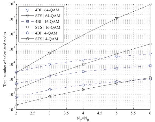
Fig. 6. Total number of calculated nodes depending on antenna number and modulation scheme. Maximum survivor node number  $k=4$ , SNR=10dB. Single Tree Search (STS) is compared to improved  $k$ -best algorithm (KBI).
