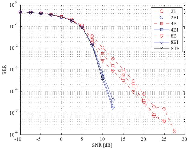
Fig. 4. Bit Error Ratio (BER) of 64-QAM system with  $N_T = N_R = 4$ . Single Tree Search (STS) is compared to  $k$ -best (KB) and improved  $k$ -best algorithm (KBI) using different  $k$ -values of maximum survivor nodes.
