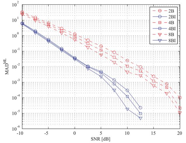
Fig. 3. Mean Absolute Deviation (11) between true ML distances (by STS) and approximated ML distances (by KB, KBI) with different  $k$ -values of maximum survivor nodes. 64-QAM system with  $N_T = N_R = 4$ .
