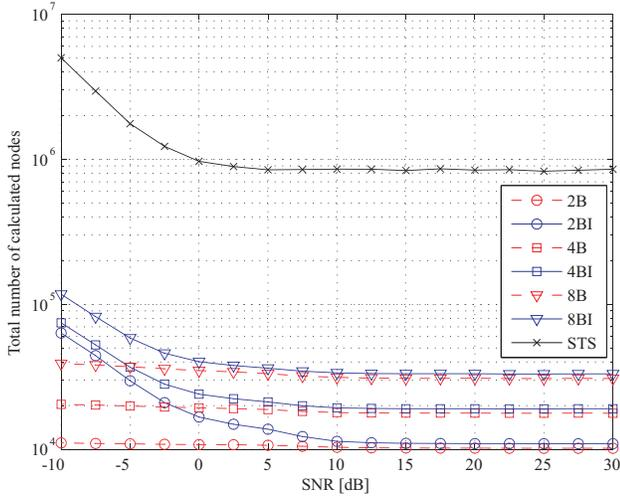
Fig. 5. Total number of calculated nodes using 64-QAM system with  $N_T = N_R = 4$ . Single Tree Search (STS) is compared to  $k$ -best (KB) and improved  $k$ -best algorithm (KBI) using different  $k$ -values of maximum survivor nodes.
