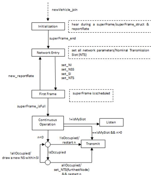
Fig. 1. STDMA algorithm implemented
