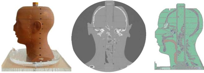
Fig. 3: From left to right: MATROSHKA ground phantom head, CT-scan of the same phantom and the phantom's voxel geometry MATSIM-Head for input in the FLUKA Monte Carlo code.
