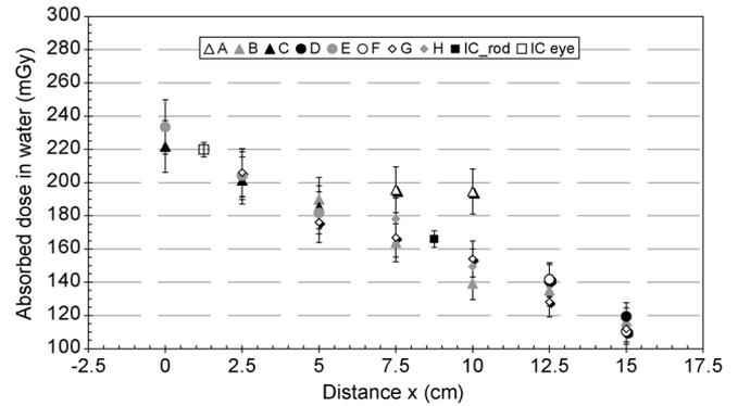
Fig. 6. Measurements of absorbed dose in water,  $D_W$ , due to  $^{60}\text{Co}$  mono-directional irradiation (MATROSHKA head slice #4; TLDs within tubes A-H and IC measurements in central rod slice #2 and eye box slice #3).
