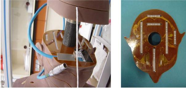
Fig. 1. Left: Inside view of the MATROSHKA phantom head (slice #3) housing active and passive eye detectors. Right: Cut through the head (slice #2) with passive TLDs. (Credit DLR).
