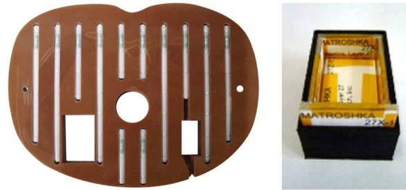
Fig. 2. Left: passive TLDs in the intestine (slice #27) and cut outs for active and passive organ dose boxes. Right: typical design of an organ dose box used for passive detectors. (Credit DLR).
