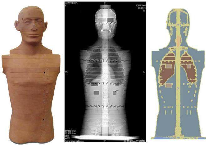
Fig. 4: From left to right: MATROSHKA phantom torso, computer tomography of the phantom and the phantom's voxel geometry MATSIM-Torso v1.1, for input in the FLUKA Monte Carlo code.
