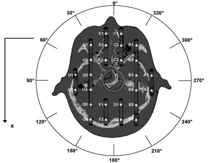
Fig. 5. Irradiation set-up of the MATROSHKA phantom head and TLD position coding in slice #4.
