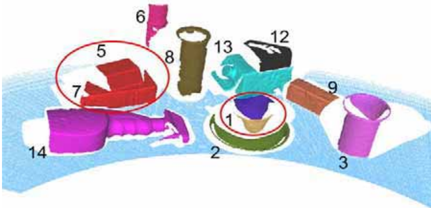
Fig. 5. Results after the first segmentation step. Object no. 1 is cut into two parts and objects no. 5 and 7 are overlapping. The not perfectly segmented objects are red encircled
