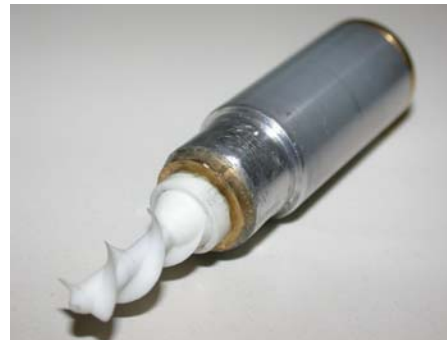
Figure 1: Prototype of the pump on a scale of 2:1, housing of pumping unit removed.
