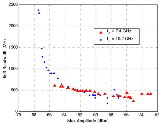
Fig. 5. The 6dB bandwidth of the random pulse stream versus received maximal amplitude.
