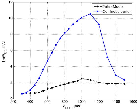
Fig. 2. Current consumption comparison for an unmodulated continuous carrier and pulse modulation.
