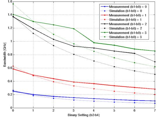
Fig. 3. Simulated and measured bandwidth created by the adjustable pulse width.
