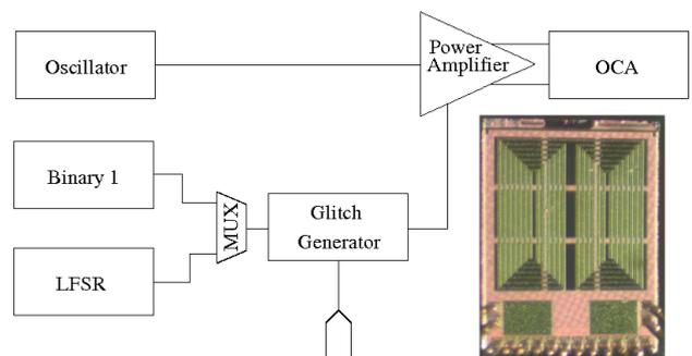
Fig. 1. Basic Diagram of the ultra wideband pulse amplitude transmitter, featuring a microscopic picture of the active UWB RFID tag manufactured in 130 nm CMOS.
