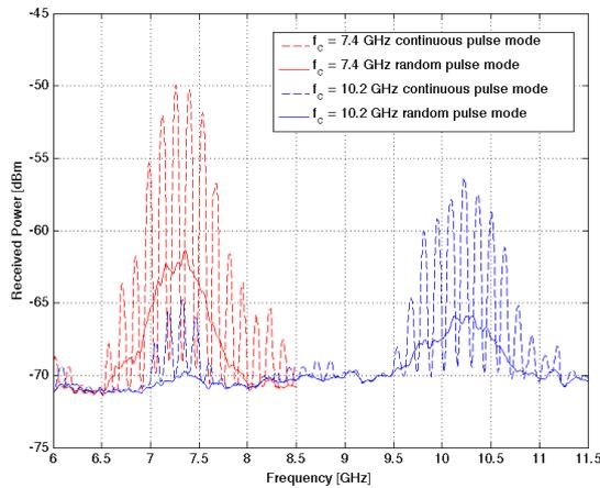
Fig. 4. Random and continuous pulse mode radiated by the coil on-chip antenna at 7.4 GHz and 10.2 GHz.
