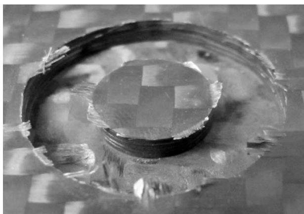
Fig. 1. Fraying and delamination
