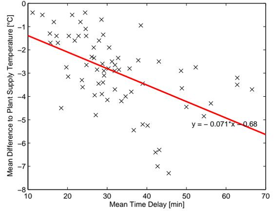
Figure 4: Temperature loss against transport time delay.
