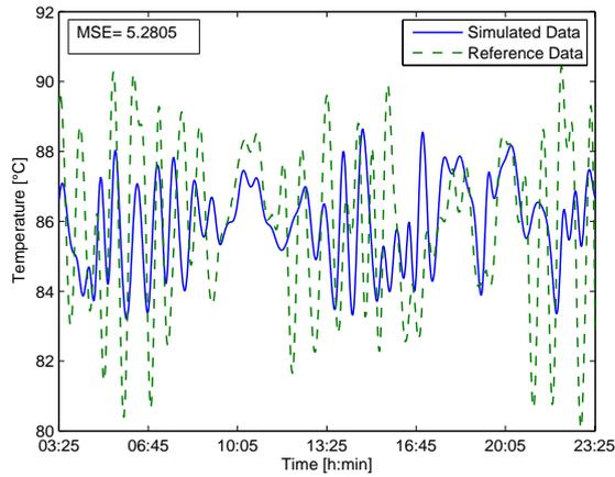
Figure 9: Simulated and reference supply temperature profile at consumer 1.
