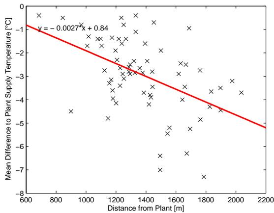
Figure 3: Temperature loss against distance.
