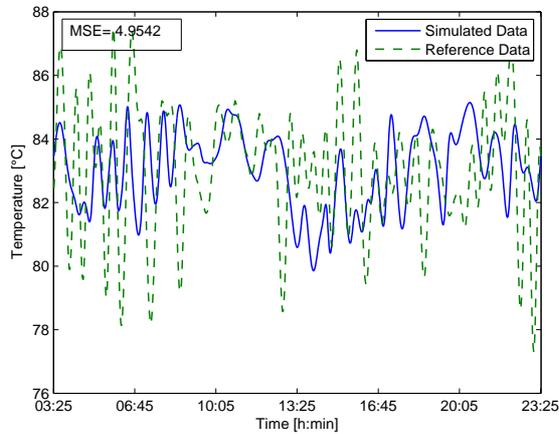
Figure 10: Simulated and reference supply temperature profile at consumer 2.
