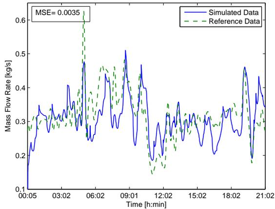
Figure 6: Simulated and reference mass flow rates for consumer 2.
