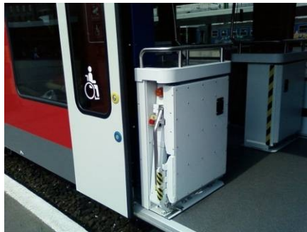
Fig.5. Stowed lift at Stadler train (Hungarian Railways)
