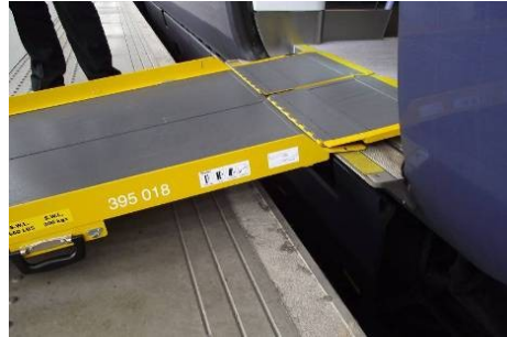
Fig. 3. Ramp fixing example Fig.4. Ramp with raised edges in contrast colours
