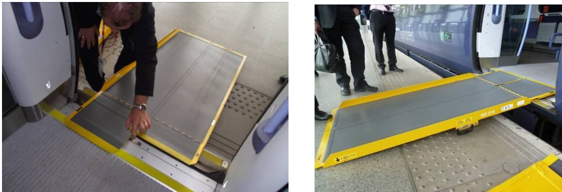
Fig.8: Manual mobile Ramp (Port-a-Ramp, UK), bridging the gap between the train and the platform (South Eastern Trains, England)
