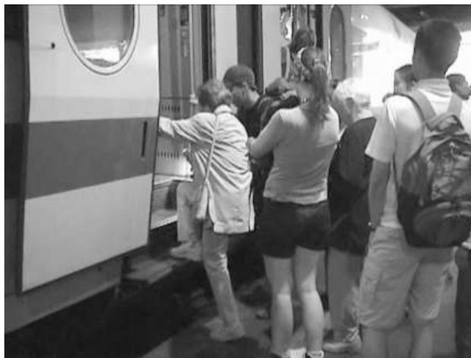
**Fig. 1** *Boarding passenger onto an ICE on a platform height of 38cm*
