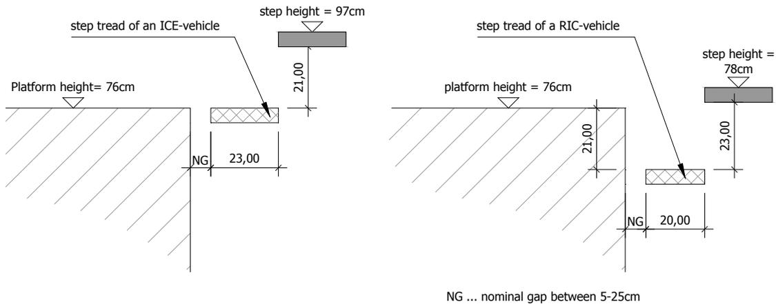
**Fig.2** Gap between an ICE and platform with a height of 76cm (left)
